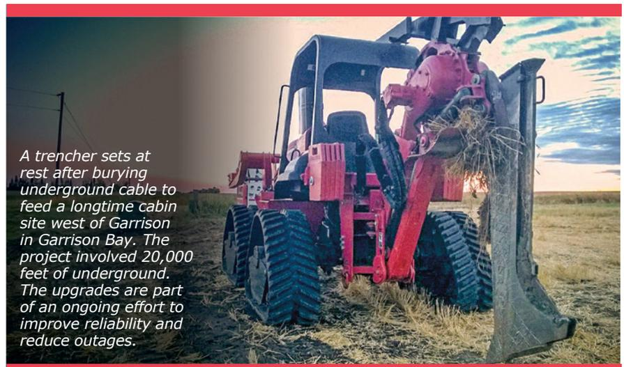
*A trencher sets at rest after burying underground cable to feed a longtime cabin site west of Garrison in Garrison Bay. The project involved 20,000 feet of underground. The upgrades are part of an ongoing effort to improve reliability and reduce outages.*
